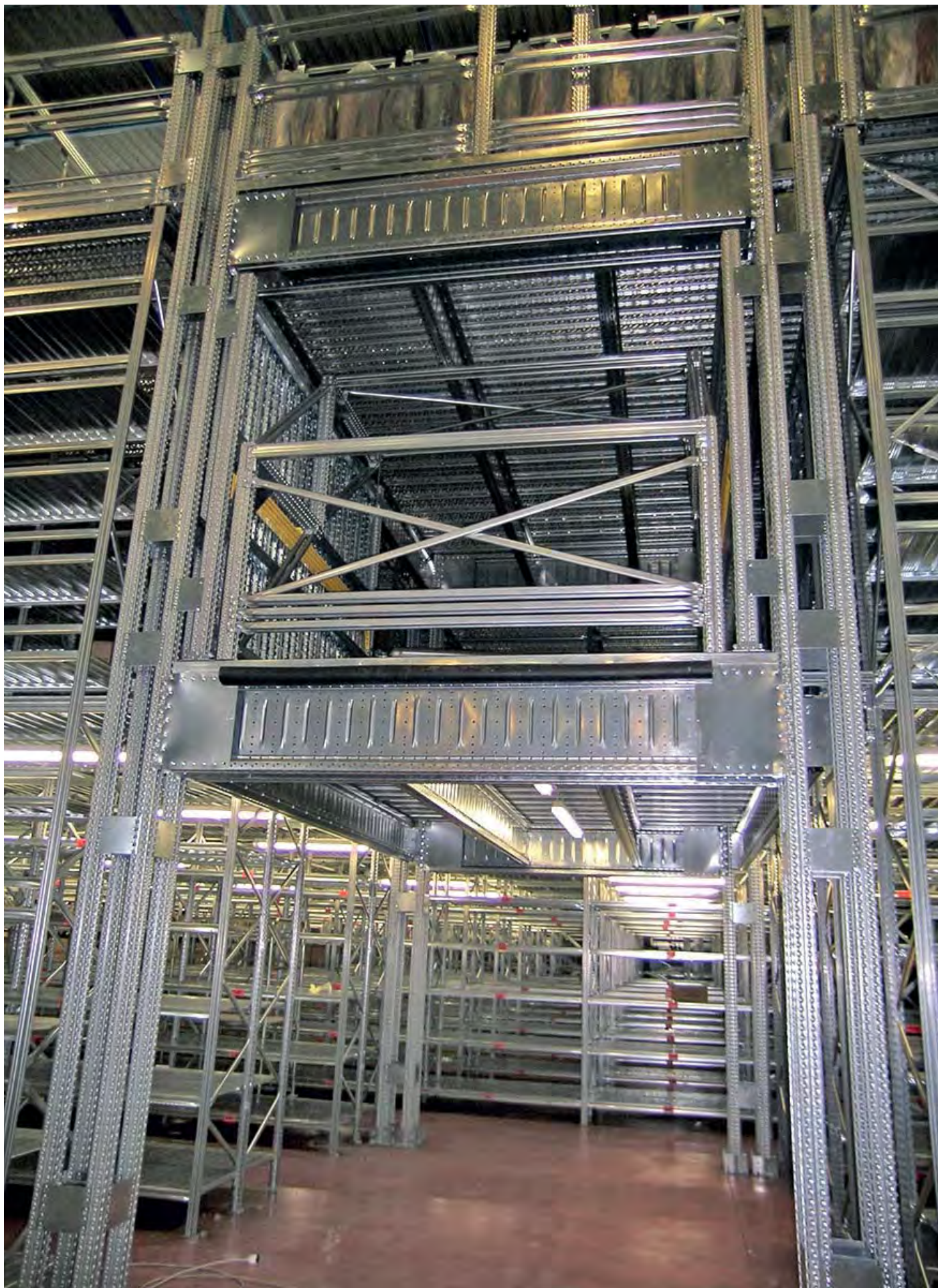
Modular METALSISTEM multi-tier installation and mezzanine made from METALSISTEM's UNIRACK and SUPER-6 product series
