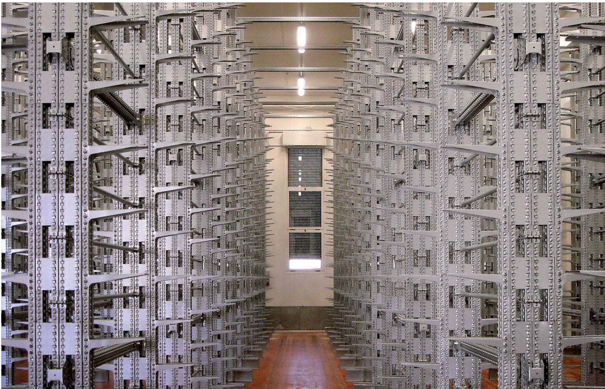
METALSISTEM Seismic Racking Structure designed for a Dairy Factory - High Density Storage of Parmesan Cheese
