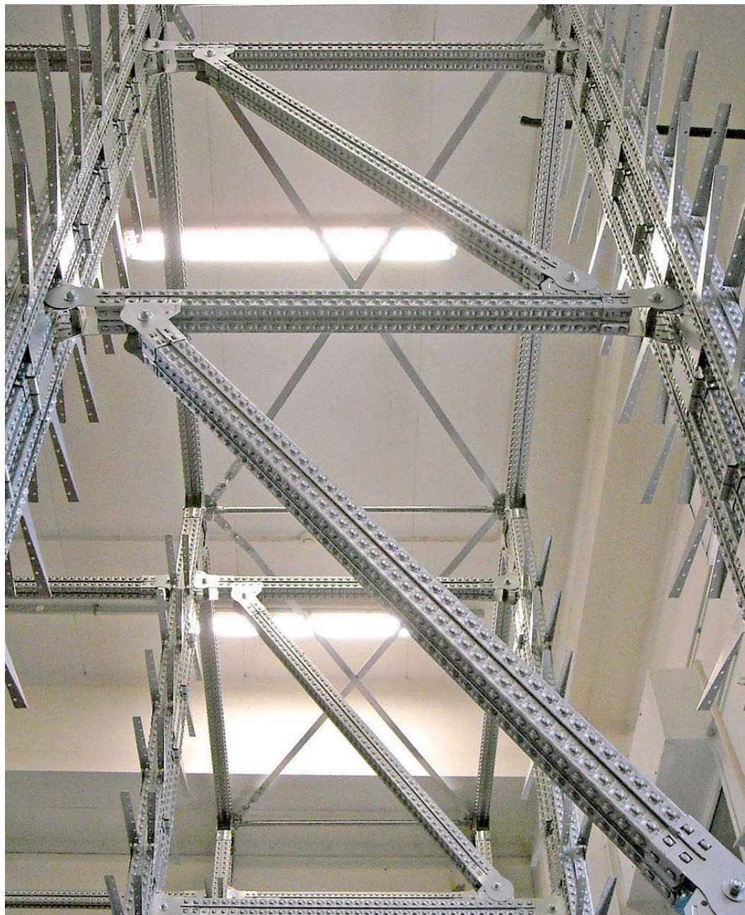
METALSISTEM Seismic Racking Structure designed for a Dairy Factory - High Density Storage of Parmesan Cheese <October 2012>
